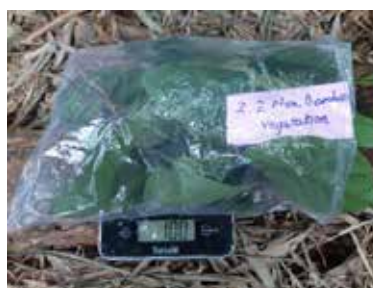
Use precision electronic scale to weigh fresh mass of sample
