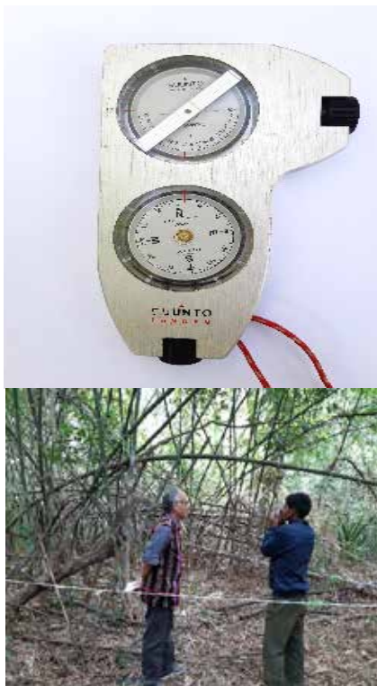
Figure 42. Suunto and LaserAce equipment to measure H (left to right, respectively) (Photos: Bao Huy, 2019).
