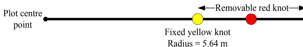
Figure 33. Knotted rope for a circular plot of 100 m 2 with a yellow knot at a radius of 5.64 m and add one more removable red knot to lengthen the radius of the plot on the slope.
