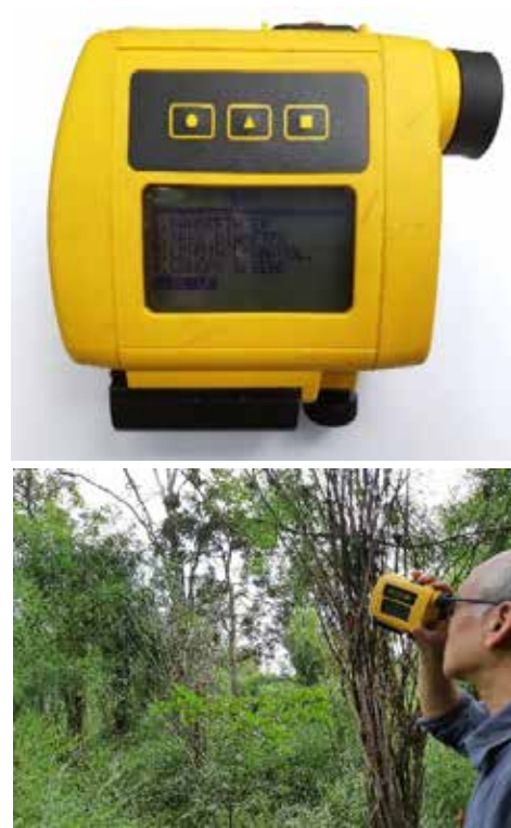
Figure 42. Suunto and LaserAce equipment to measure H (left to right, respectively) (Photos: Bao Huy, 2019).
