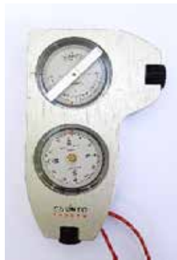
Figure 34. Suunto Clinometer, obtaining a slope using the clinometer (left to right, respectively) (Photos: Bao Huy, 2019).
