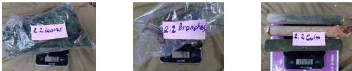
Figure 7. Samples of leaves, branches and culms are weighed using a precision electronic scale on site and brought to the laboratory to determine the fresh-to-dry mass ratios (Photos: Bao Huy, 2019).
