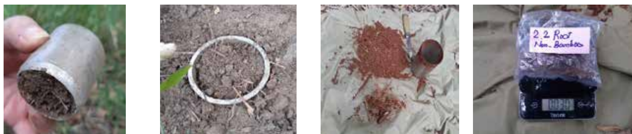
Figure 46. Soil core; using the soil core to take soil samples and roots of plants (Photos: Bao Huy, 2019).
