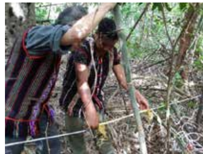
Figure 35. Using knotted ropes to establish a circular plot and adding extra radius distance to the slope (left to right, respectively) (Photos: Bao Huy, 2019).
