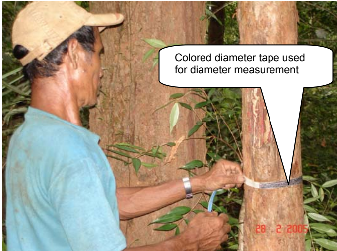
Illustration 7: Use of simple inventory tools as the colored diameter tape for resource assessment
