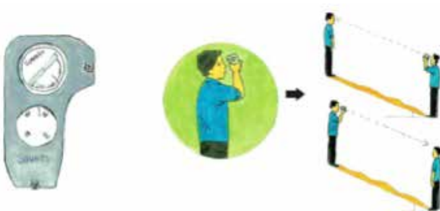
Figure 3. Compass and clinometer and obtaining slope using clinometer
