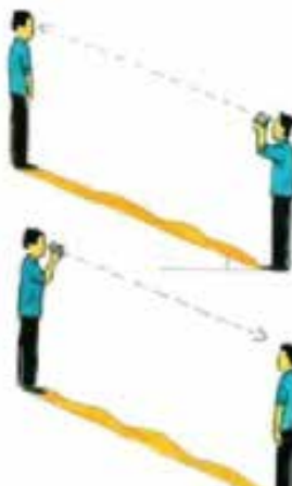
Figure 8. Obtaining slope using clinometer
